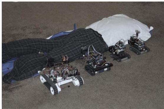
Fig. 15 – Human Rescue using four UB swarm robots.
