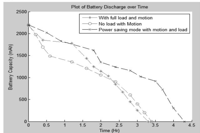
**Fig. 7 – Battery Capacity Vs Operating Time for Rover 1.**
