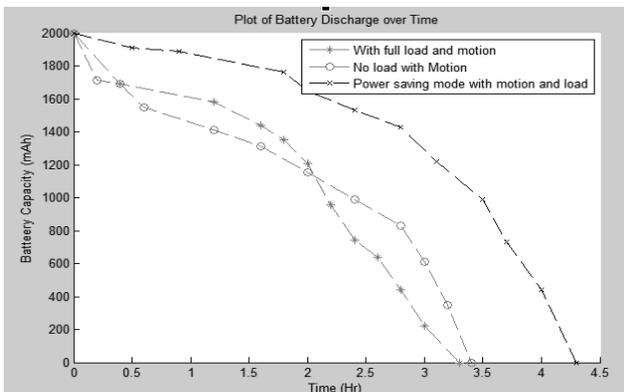
**Fig. 11 – Battery Capacity Vs Operating Time for Rover 5.**
