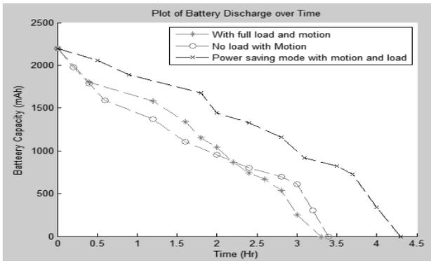
**Fig. 8 – Battery Capacity Vs Operating Time for Rover 2.**
