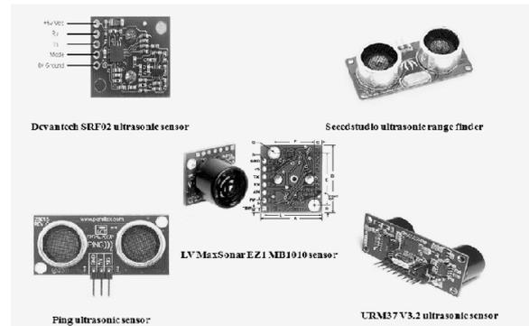
Fig. 2 – Ultrasonic Sensors used in UB Swarm.
