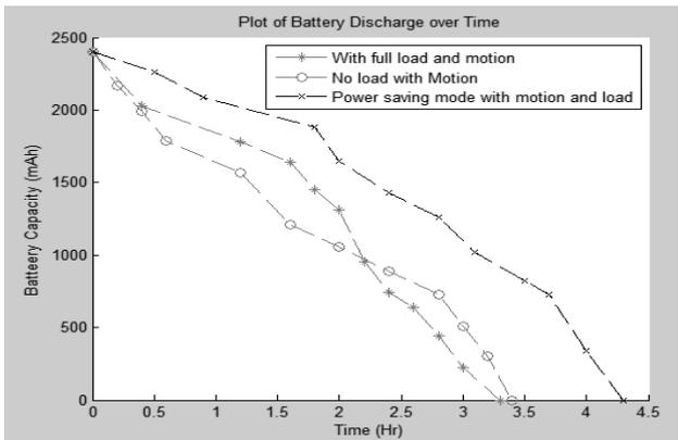
**Fig. 9 – Battery Capacity Vs Operating Time for Rover 3.**
