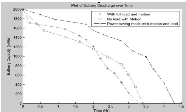
**Fig. 10 – Battery Capacity Vs Operating Time for Rover 4.**
