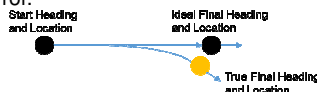
Figure 7: Accumulating PI error in a mobile robot and as seen with the ratbot .
